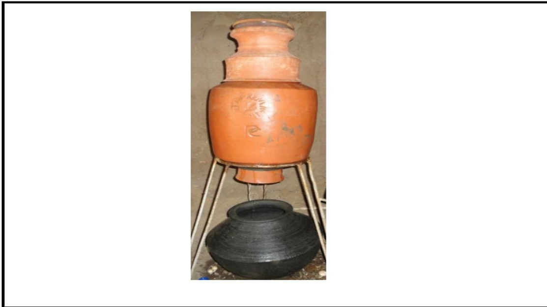
Figure 1: Final product of INREM's filter on location in Jhabua
